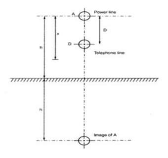
Fig.2.19 The potential of point A with respect to the earth is given by,
