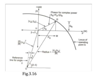
An increase in power delivered means that point G will move along the circle until the angle  $\beta - \delta$  is zero. Thus so long as  $\delta = \beta$ , maximum power is delivered. With further increase in  $\delta$ , results in less power at receiving end. The equation for maximum power is given by,
