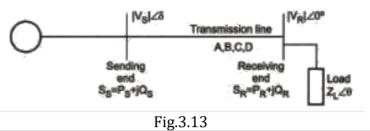
The complex power delivered by the receiving end and that received by the sending end of the transmission line is given as,
