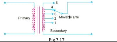
(a) Off load tap-changing transformer. Fig. 3.17. shows the arrangement where a number of tappings have been provided on the secondary. As the position of the tap is varied, the effective number of secondary turns is varied and hence the output voltage of the secondary can be changed. Thus referring to Fig. 3.17, when the movable arm makes contact with stud 1, the secondary voltage is minimum and when with stud 5, it is maximum. During
