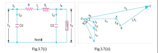
The \*phasor diagram for the circuit is shown in Fig. 3.7(ii). Taking the receiving end voltage as the reference phasor, we have,
