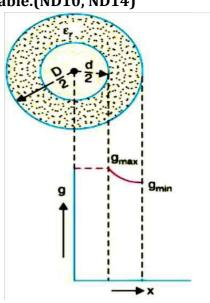
By definition, electric intensity is equal to potential gradient. Fig 4.24 Therefore, potential gradient g at a point x meters from the Centre of cable is
