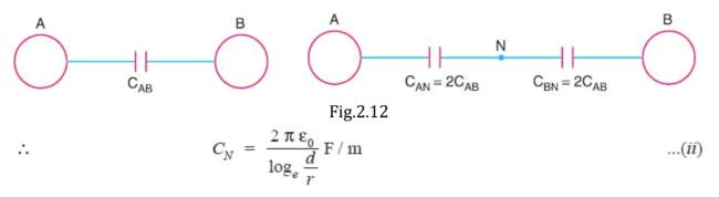
The reader may compare eq. (*ii*) to the one for inductance. One difference between the equations for capacitance and inductance should be noted carefully. The radius in the equation for capacitance is the actual outside radius of the conductor and not the GMR of the conductor as in the inductance formula. Note that eq. (*ii*) applies only to a solid round conductor.
