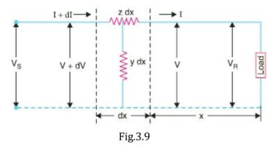
Consider a small element in the line of length dx situated at a distance x from the receiving end.
