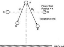
Consider the loop formed by the conductors A and D. Let the radius of each power line conductor be r. Let the distance between conductors A and D be whereas the distance between conductors A and E be D<sub>2</sub>. Assuming that in loop AD, A is contributing to the e.m.f. induced in D. If we neglect the internal flux linkages then the inductance of this loop is given by,
