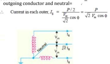
Current in neutral\* wire =  $\sqrt{I_8^2 + I_8^2} = \sqrt{2}I_8$ Assuming the current density to be constant, the area of X-section of the neutral wire will be  $\sqrt{**}$  times that of either of the outers.
