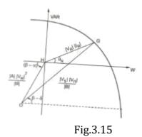
It can be shown that for constant values of VR and Vs and for variable values of IR the point G moves on a circle with centre O
