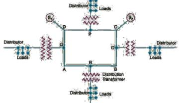
Distributors are connected to points *O*, *P*, *Q* and *R* of the feeder ring through distribution transformers.
