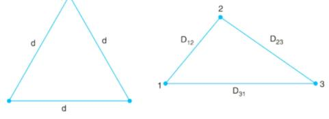
Inductance/phase/m =  $10^{-7} (0.5 + 2 \log_e d/r) H$ =  $10^{-7} (0.5 + 2 \log_e 200/0.62) H$ =  $12 \times 10^{-7} H$ Inductance/phase/km =  $12 \times 10^{-7} \times 1000$ =  $1.2 \times 10^{-3} H = 1.2 \text{ mH}$
