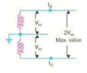
Max. voltage between conductors =  $2 V_m$
